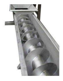
Trough - U Type Screw Conveyor is continuous conveying equipment which used to transport powder, granular and dry bulk materials. It consists of bearing seat, screw blade, screw shaft, hang bearing, conveyor casing and driven device, etc. Single or combination of multiple screw equipment can be used to integrate with each other to meet particular on-site requirements. It has trough type tube with multiple inlets and outlets.
